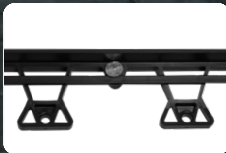
SPIKES CAN GO ANYWHERE IN BETWEEN THE CUT BRACE AND EDGING WALL WHICH HELPS TO DIMINISH EDGE PULL AWAY WHEN INSTALLING.
